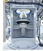
Maintenance flap at the pressur chamber
