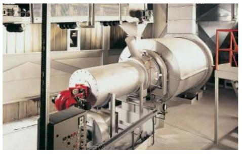
Careful material treatment The material is treated with care. It will not overheat due to the uniflow principle.
