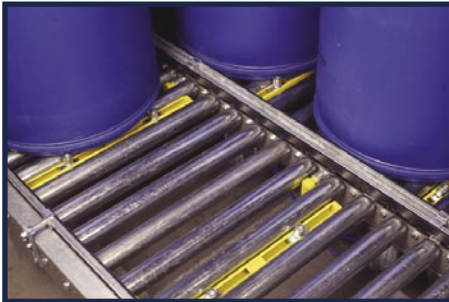
■ Stop dog for stopping or separation
