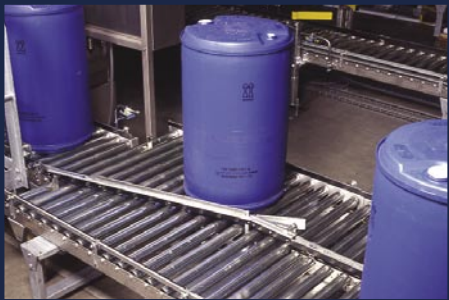
■ Filled drum feeding with pivoting diverter
