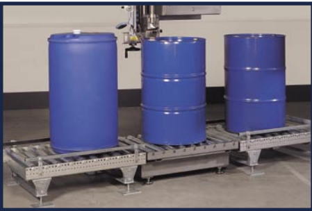
■ Non-driven drum roller for semi-automatic system
