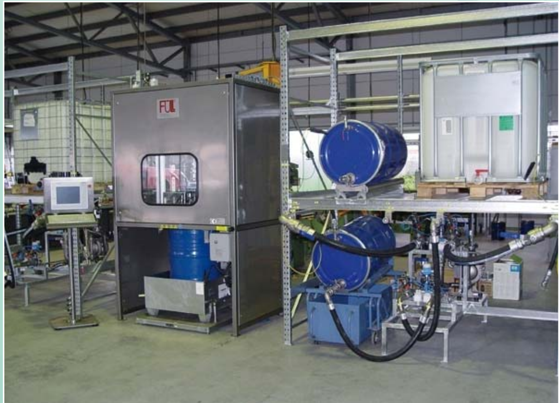
Batch supply of lamination components with integrated agitator for the supply of a lamination machine.
