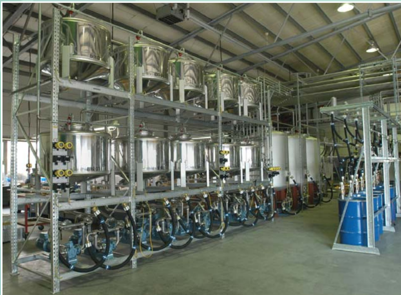
Combination of 1 m 3 - to 5 m 3 -tanks and 200 l-barrels for the storage of pastes, additives and basis
