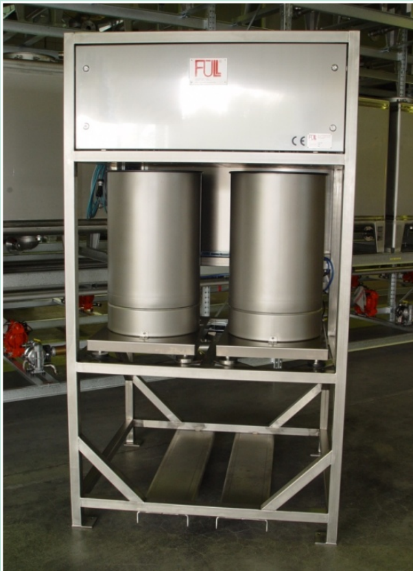
Double unit for semi-continuous supply of lamination components into a lamination trough
