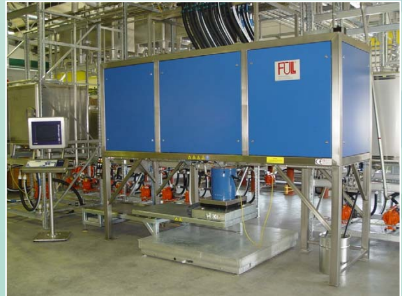
FS 182 - with 1.500 kg-floor scale and 60 kg-scale
