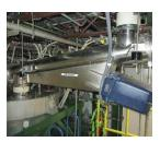
Vibrating conveyor up to 400 t/h and up to 10 mm grain size Vibrating conveyor tube up to 100 t/h and up to 10 mm grain size
