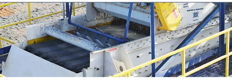
The Niagara L-Class vibrating screen is a versatile and easy to maintain linear machine, with no timing belts or gears that need replacing.
