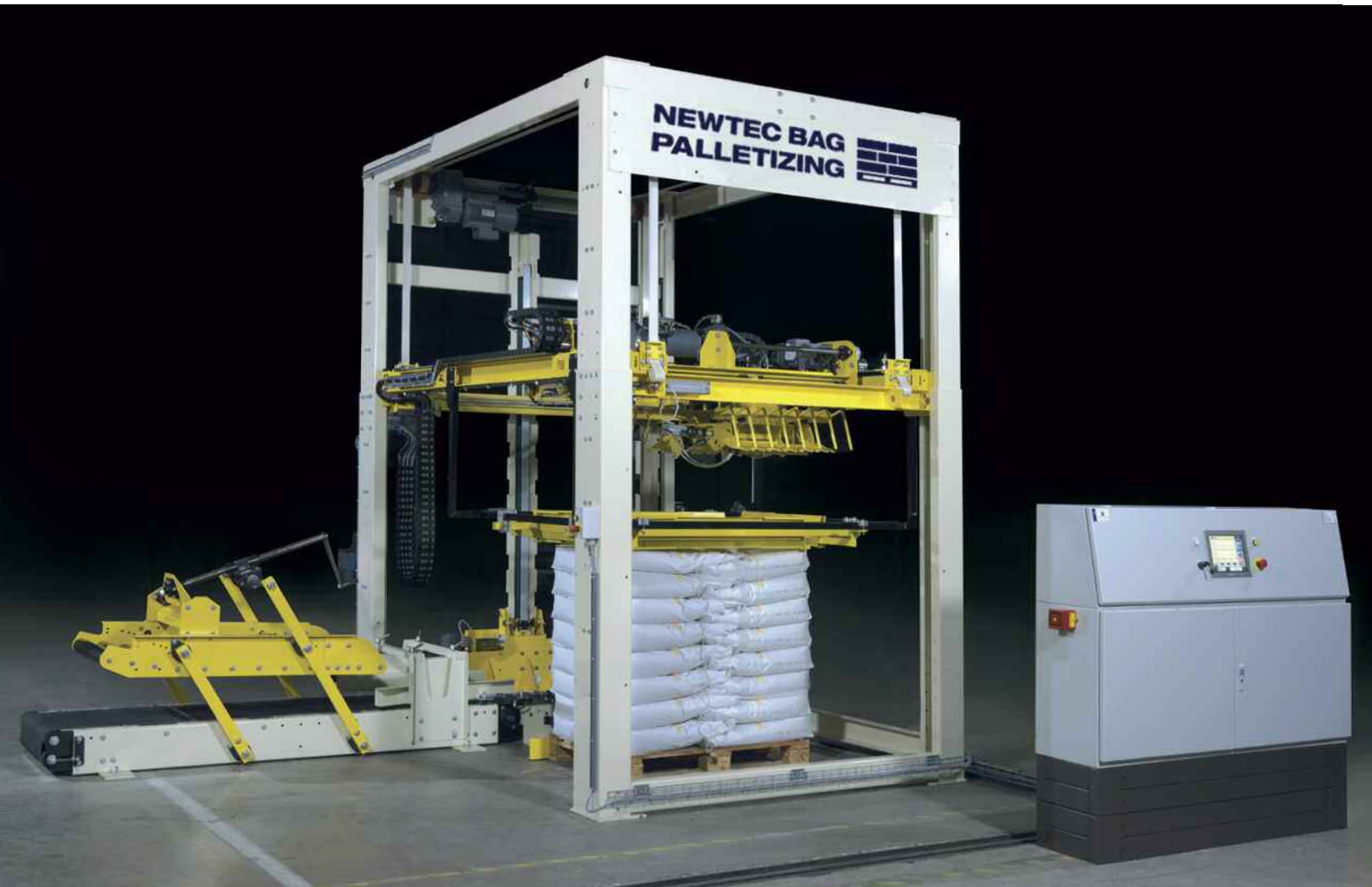
The palletizer - G 300 series - is designed for low capacities of up to 300 bags/hr of 5 to 50 kg.
