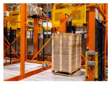
▲ Empty pallet feed MSK conveyor systems also fully automatically feed empty pallets to the sheeter.
