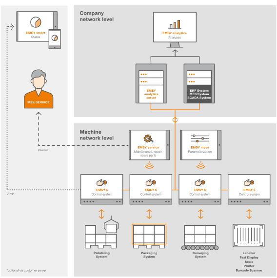
Information from all kinds of peripheral devices is managed by the software and can be forwarded to your system (MES. ERP, SCADA, etc.).
