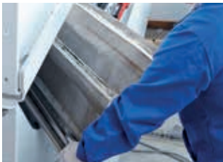
02:30 min Installation of a new screen cloth.
