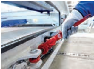
02:45 min The screen cloth is tensioned once again with quick-action fasteners.
