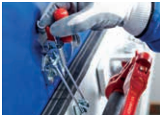
05:00 min The maintenance doors are closed and dust-proof the screen cloth and screen box at the sides.
