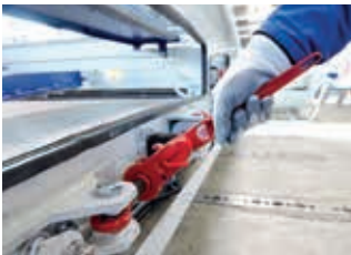
00:40 min The screen cloth is tensioned by rapid-action fasteners.
