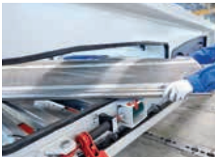
02:15 min The screen cloth can be installed and removed in a space saving manner.
