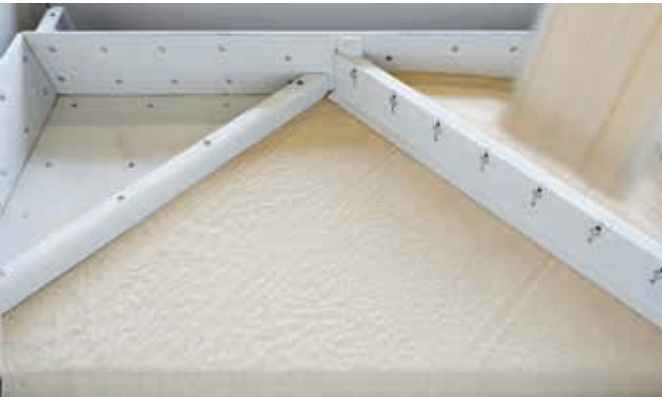
The feed material is distributed across the full width of the screen cloth.
