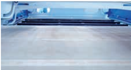
Optimally tensioned sandwich woven screen.
