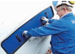
00:00 min The maintenance doors at the defective screen cloth are opened on both sides.
