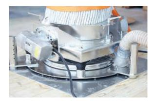
The Haver R-Class is a reject screening machine. It has been developed in a compact design and especially for fully automatic screening, upgrading well-known Big Bag and silo systems. The use of HAVER R-CLASS guarantees that no reject or agglomerates will get into the final product at the packing process.
